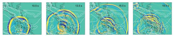
Figure 9. Time-snapshots of simulated ver. motion. Thin white lines are contours of basin V<sub>P</sub> model structure at 500 m depth.
