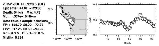
Figure 5. Focal mechanism solution computed based on CNSN broadband data. Best double couple solutions (nodal fault planes) are reported as FP1 and FP2.
