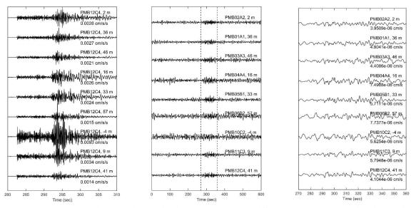
Figure 4. Vertical-comp. acceleration (left) and velocity time-series (middle) from IA stations are band-passed filtered with corners of 0.1 & 0.5 Hz. The right panel shows zoomed-in window (depicted with dashed lines in the middle panel). The name of stations, their depth of recordings, and peak ground velocity (PGV) values are reported on each trace.
