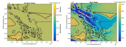
Figure 2. Depth slice(s) of non-basin and the updated basin Vp models from surface to 250 m. Thin black lines are coastlines and thick contours (5.5 km/s) representing the basement of the basin. Modified after Molnar (2011).
